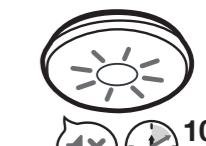
Combination smoke and CO alarms can react to cooking fumes or other non emergency situations. Your alarm features Silence technology. In the event of a known false alarm you can temporarily silence it by pressing the Test / button. Your alarm will automatically return to full sensitivity after 10 minutes.
