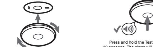
2c Press the Test / button. The alarm will sound a reduced alarm volume.
