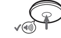
Press and hold the Test button for 10 seconds. The alarm will sound the full alarm volume.
